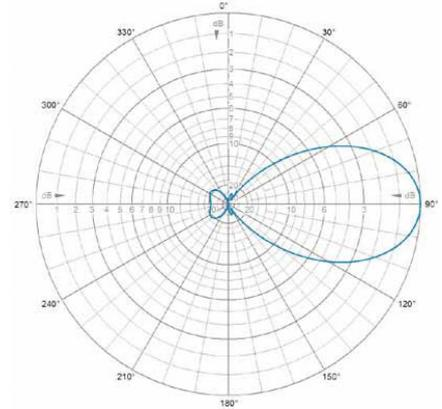
If the antennas are mounted for vertical polarization, these curves show the radiation patterns in the vertical plane.
