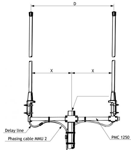
Antennas should be mounted symmetrically in relation to the mast.
