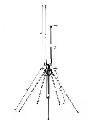
The radiator is measured from its free end to the bottom of the black insulator, while the radials are measured from their free ends to where they meet the GP-head. The radials must be placed short/long alternately.
