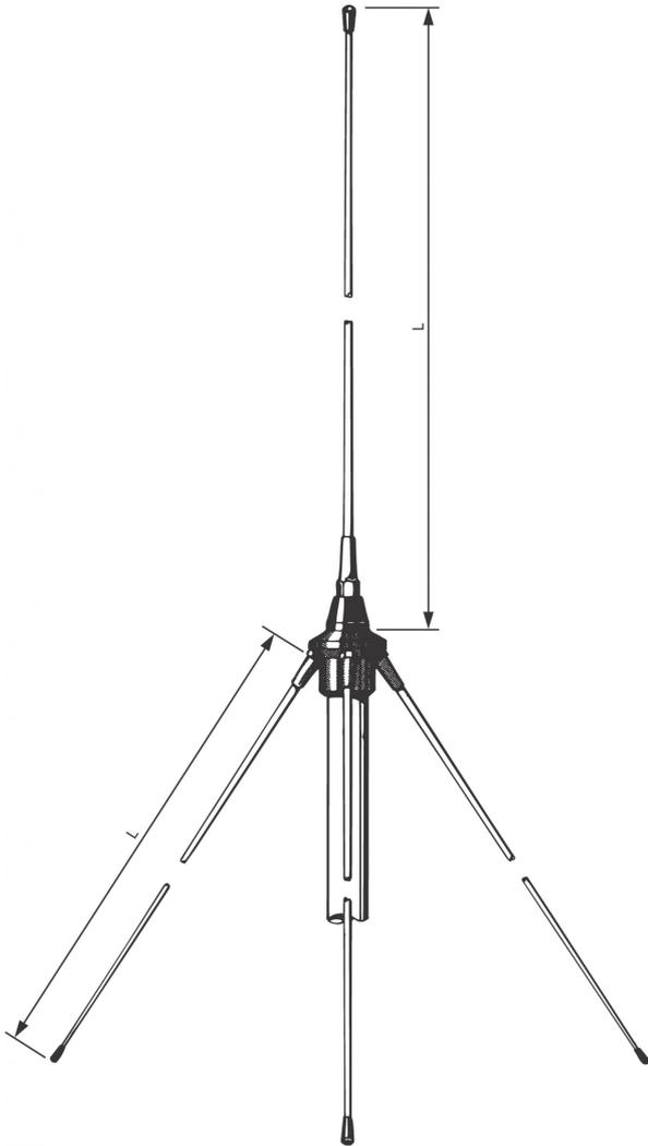
The radiator is measured from its free end to the bottom of the black insulator, while the radials are measured from their free ends to where they meet the GP-head.
